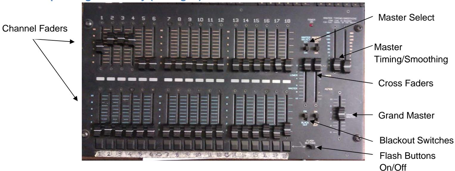
As previously mentioned, this desk can be used where “simple” lighting using only 18 ways of the Pulsar Dimmerpak is required. Basic operation allows a scene to be setup on either the top or bottom row of faders (1 – 18) with the next scene on the other row and alternating through the performance, using the Crossfade faders. Note that these faders are reversed so that in the same position one is “full” while the other is “off”.
